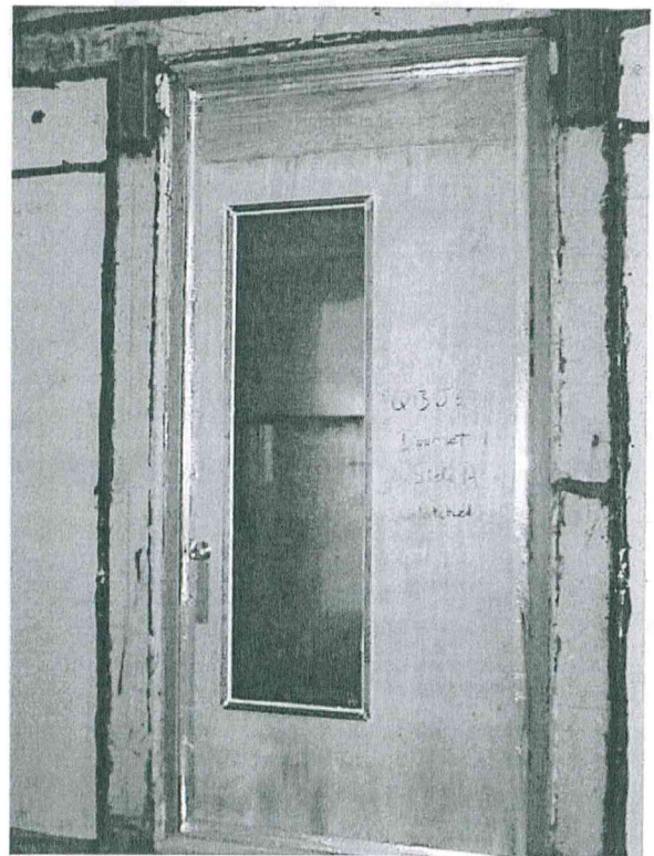
Photo 2: The unexposed face of Doorset '1' after the medium temperature test.
