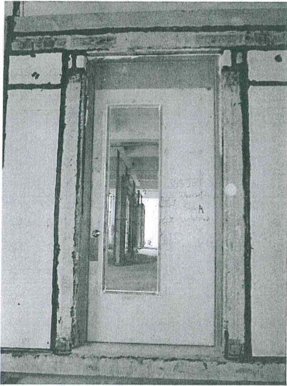
Photo 3: The exposed face of Doorset '2' before the medium temperature test.
