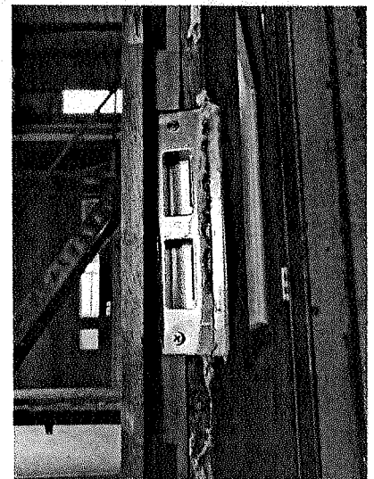
Photo 8. Strike plate position after medium temperature test.
